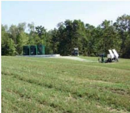
At the completion of the drilling process, the land near the finished well is restored to its original condition, as requested by a landowner. All that remains is a wellhead (called a Christmas Tree), a small amount of production equipment, measuring devices and storage tanks to collect water that returns slowly up the wellbore. Even more energy can be produced by developing multiple wells from a single drilling pad, with a minimum of earth disturbance activity.
